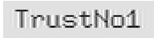
Figure 2: The same text after horizontal low-pass filtering.
